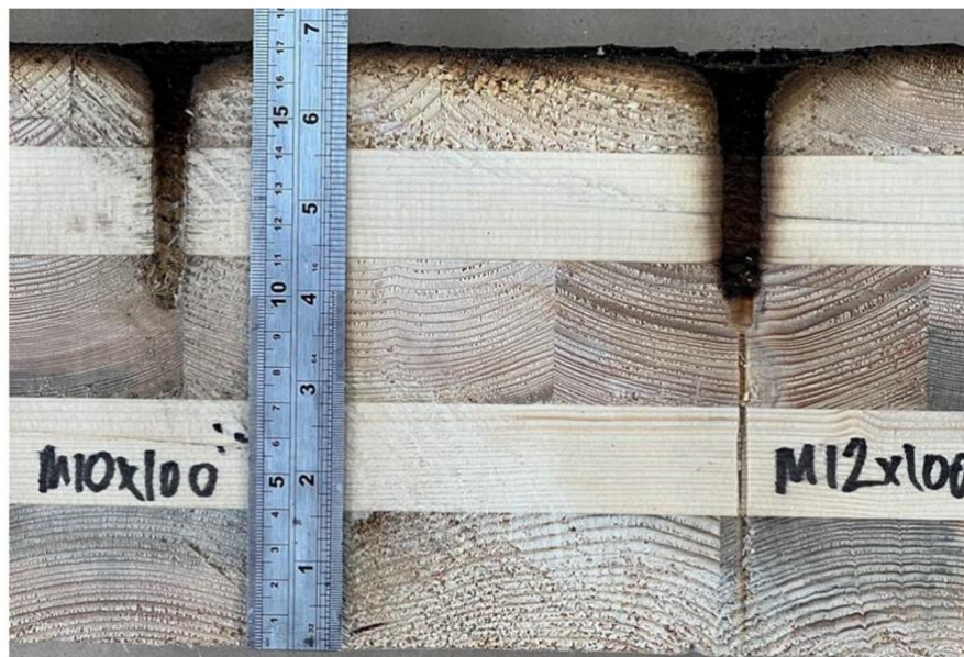
Figure 3 Post test cutaway showing heating and charring of wood around the bolt threads
