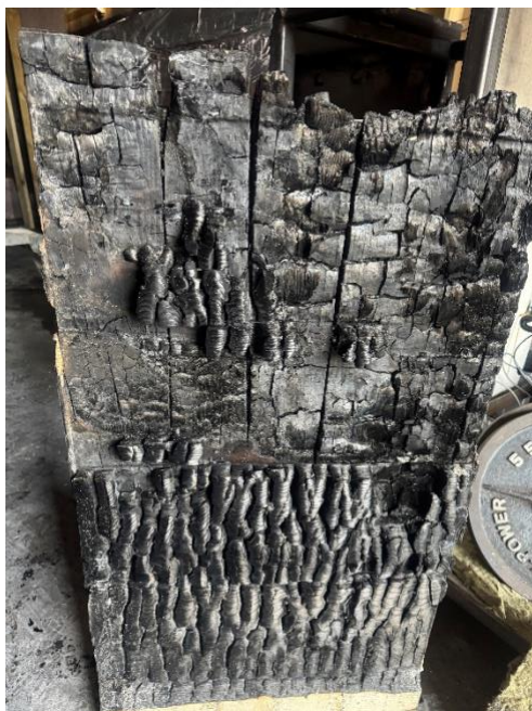
Figure 29 Wall and Ceiling samples post-test with some char cleared for measurement
