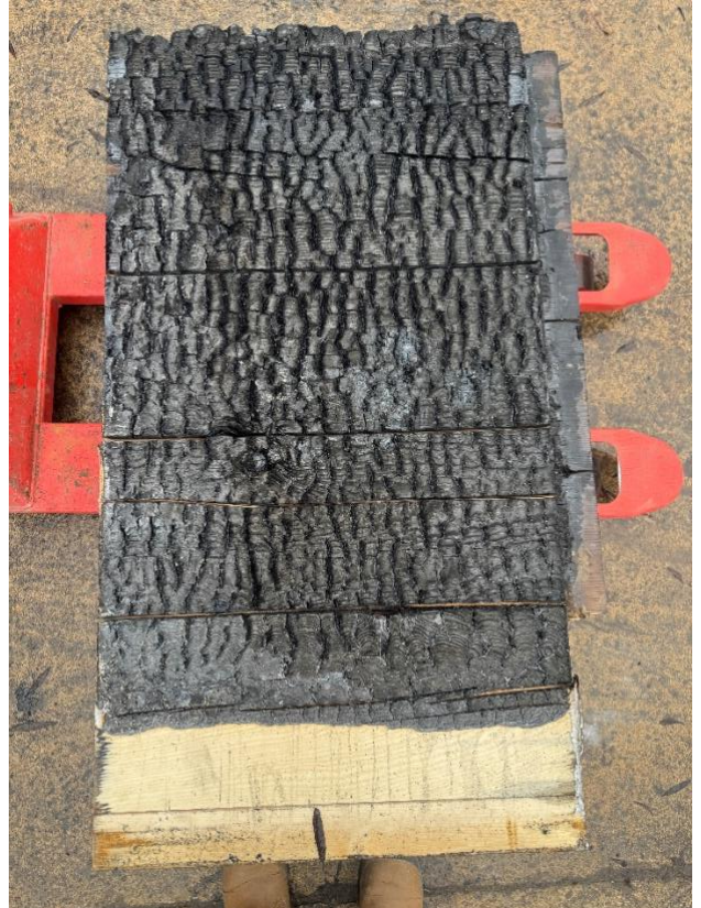
Figure 23 Wall panel post fire
