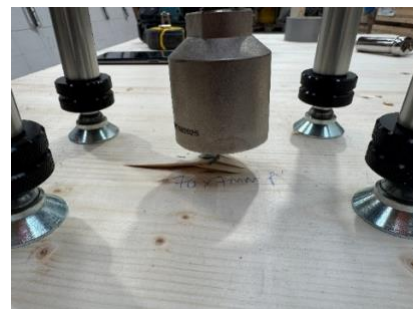
Figure 34 Load pull out close up
