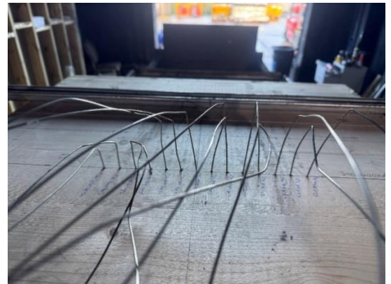
Figure 28 Position of thermocouples within the CLT for detailed thermal analysis
