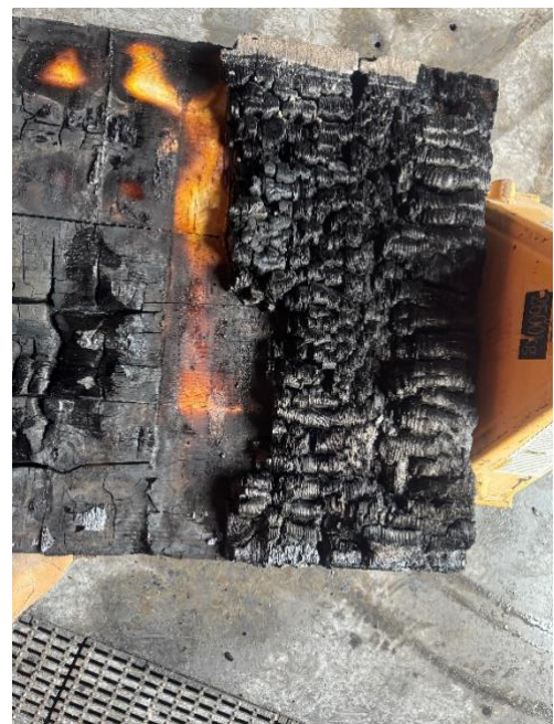
Figure 29 Wall and Ceiling samples post-test with some char cleared for measurement
