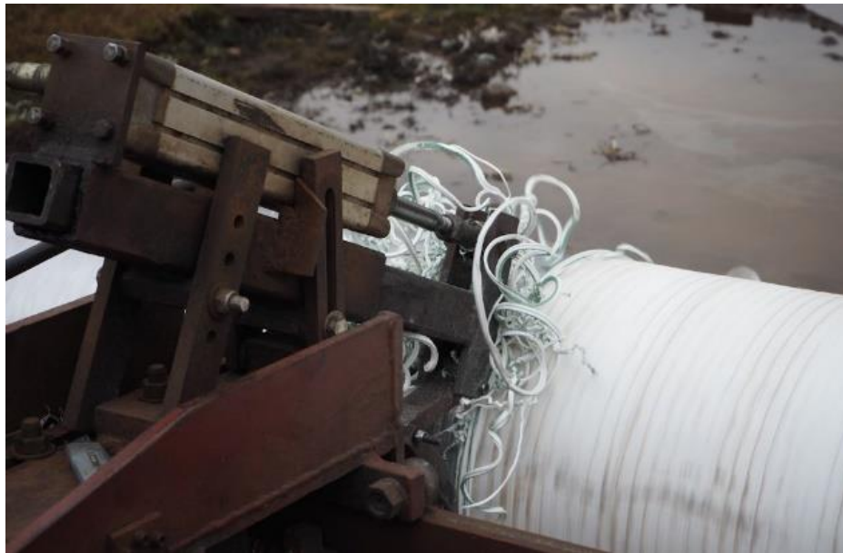
Figure 4: Plastic coating removal
