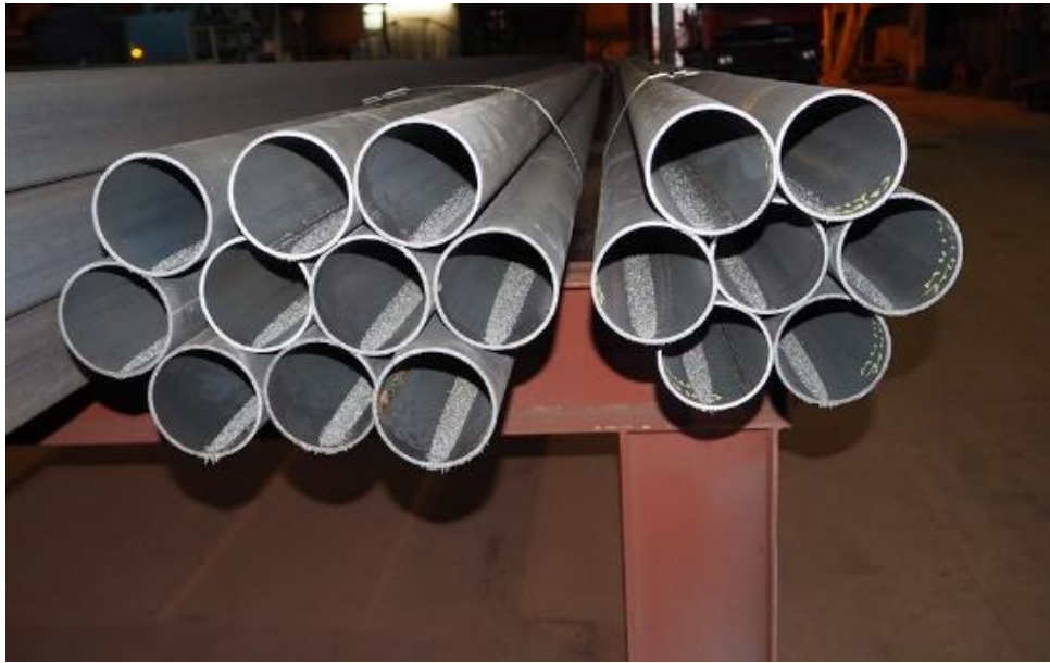
Figure 5: Shot blasted tubular.
