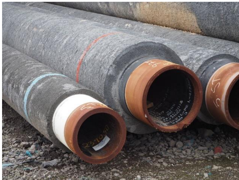
Figure 2: Concrete coated tubular
