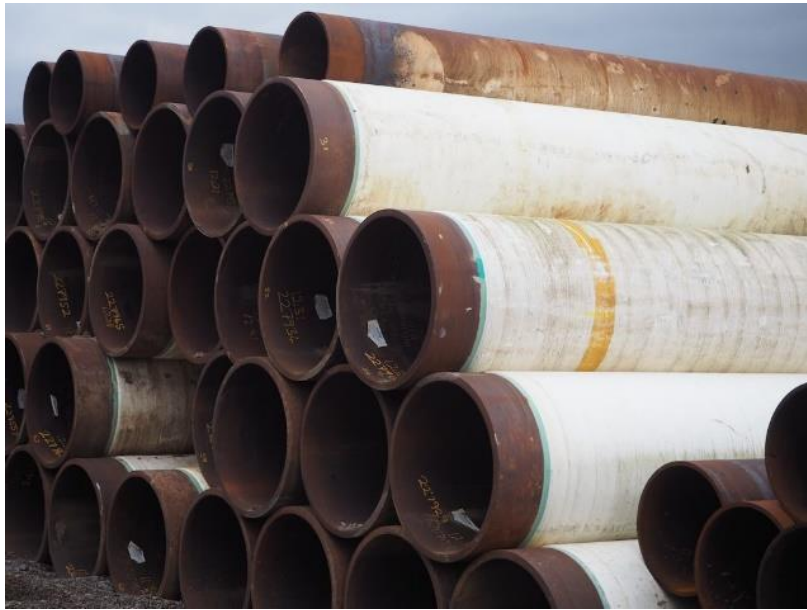
Figure 3: Plastic coated tubular
