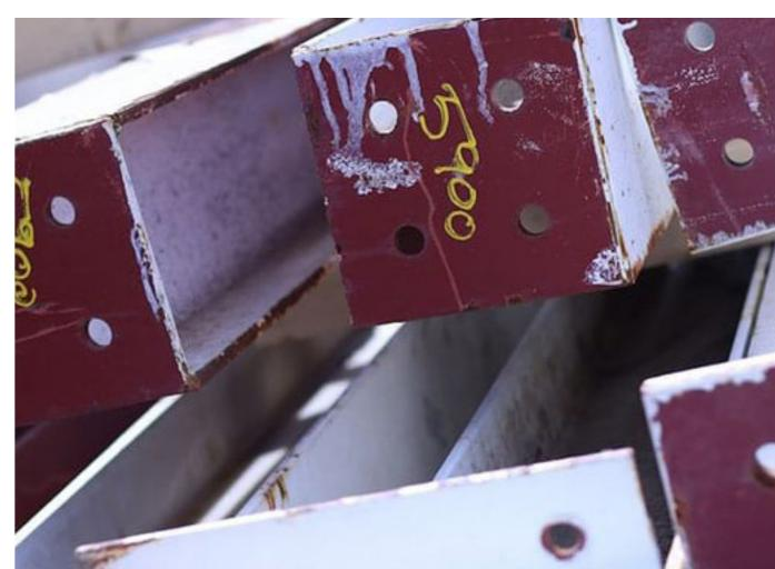
EMR Reusable Steel is more than just a reclaimed material. The care and consideration taken throughout recovery, processing and design distinguishes the EMR Reusable Steel section from the traditional alternatives.
