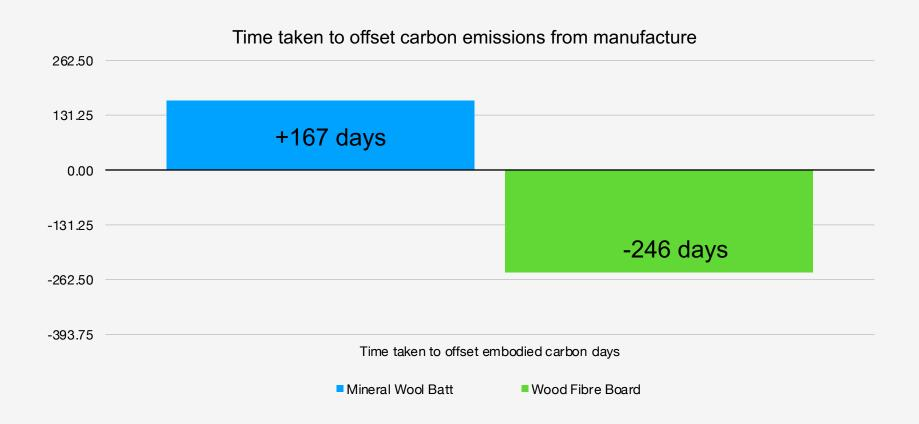
Number of days to offset carbon emissions from manufacture of insulation products. U-value  $0.29 \text{ W/m}^2\text{K}$ . Avg. Temps, Int = 18C, Ext = 5.3C
