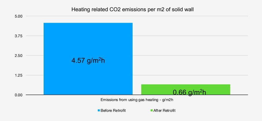
Typical gas heating related carbon emissions for a solid brick walled house with a starting U-value of around 2.0 W/m<sup>2</sup>K and finishing with 0.29 W/m<sup>2</sup>K. Avg. Temps, Int = 18C, Ext = 5.3C (Oct-Mar avg. for Midlands)
