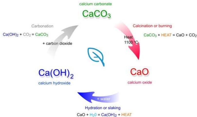
Figure 4. Lime cycle: Calcium carbonate-Calcium oxide-Calcium hydroxide.
