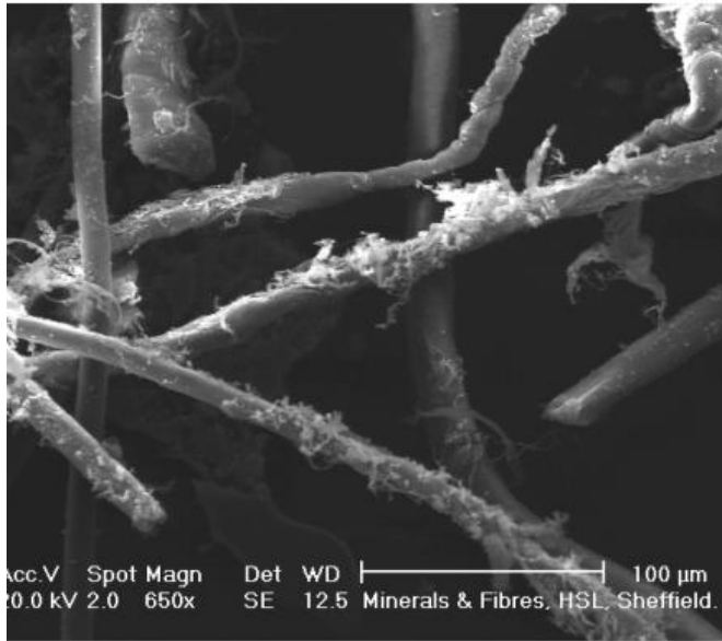
23: Large polypropylene fibres showing fibrils formed on the fibre surface
