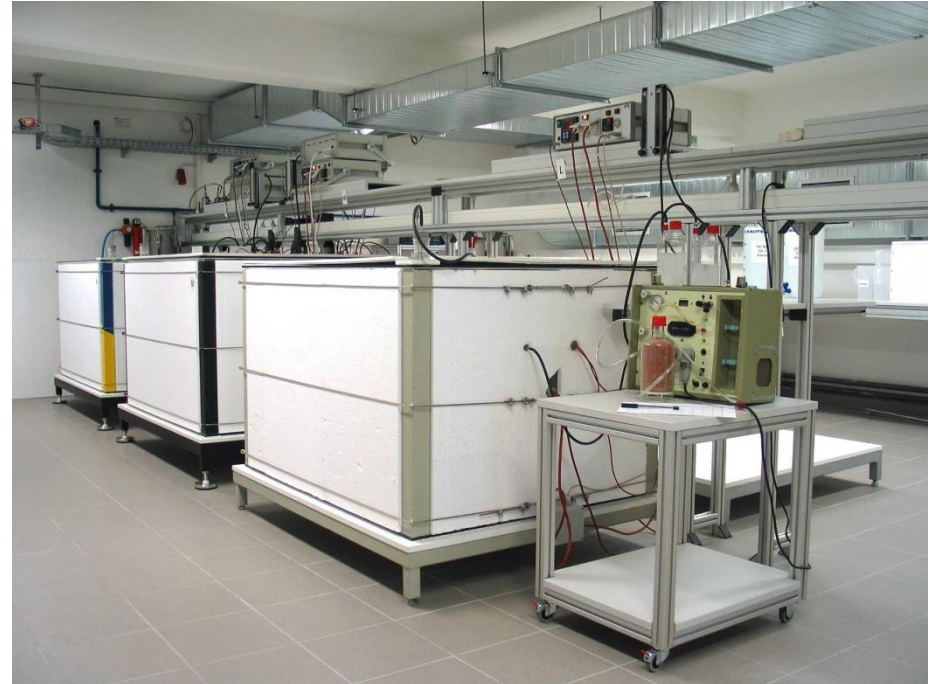
Environmental chambers for wood-based panel testing
